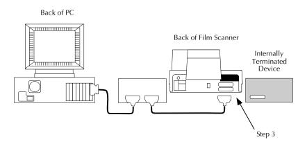
4. Attach the end of the cable you just disconnected to either of the identical SCSI ports on the back of the Scanner. Seat the connector firmly and pinch the thin wire clamps shut.
